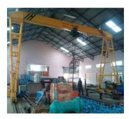
Gantry Cranes are self-propelled cranes and are useful where overhead rails cannot be installed or the movement of load is required only in specific floor area out of the whole shop floor; railings for gantry cranes are installed on the floor itself. Gantry Cranes can be either single girder or double girder depending upon load being lifted and the usage.
